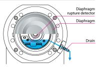
pressure caused by clogging or improper operation. A drain hole also ensures safe operation even when the diaphragm is damaged.
