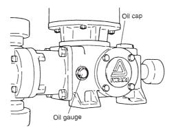
[5] Run the motor instantaneously to check for correct direction of motor rotation. The motor should run in the direction indicated with the arrow on the pump. If the direction is reversed, exchange any two wires of the three-phase power wires.
