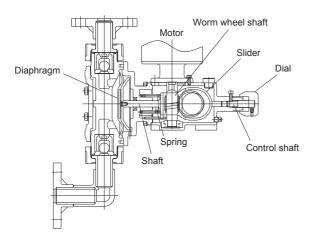
The rotation of the motor is reduced by means of the worm and wheel. The rotary motion is changed to a reciprocating motion by the spring-back mechanism (including the worm wheel shaft, slider, spring, etc.). The reciprocating motion is transmitted to the diaphragm directly connected with the shaft, changing the volume inside the pump chamber. Thus, variation of the volume inside the pump chamber and the functioning of the valves in the pump head produce pump operation.
