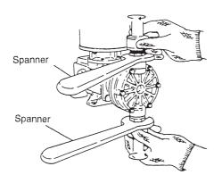
(3) When installing a LK-F 11, 21, 22, 31, or 32 flange (VC, VH, or VS type), use a spanner to fix the adapter (6) then fasten the nut (50) by hand.
