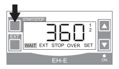
(3) Push START/STOP key to confirm the analog mode and move to WAIT mode.
