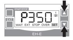
(11) Setting of stroke rate for the current value of SET point 2
