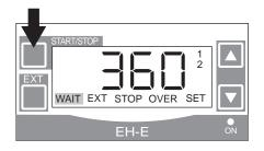
(9) Push START/STOP key to confirm the operation mode and dividing ratio.
