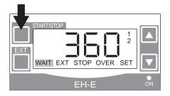
(9) Push START/STOP key to confirm the operation mode and stroke number.
