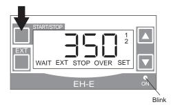
(3) Push START/STOP key to start the pump. WAIT word disappears and ON lamp blinks.
