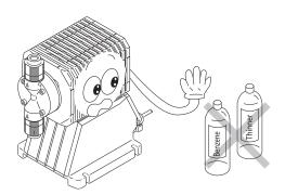
7. Do not wipe the pump body with the cloth in which is soaked by solvent such as benzene, kerosene or thinner. Otherwise, the body may be discoloured. To clean pump body, use dry cloth or the cloth in which are soaked by water or neutral detergent.
