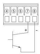
Wiring for analog input operation
