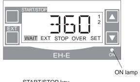
Starting and stopping pump operation
