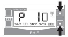
(7) Setting of stroke rate for the current value at SET point 1 Set the stroke rate for the current value at SET point 1 by ▲ and ▼ keys. Setting range is 0 - 360 spm. The pump is set at 0 spm when it is shipped from the factory.
