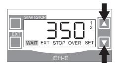
(2) Stroke rate can be changed by pushing ▲ or ▼ key at wait mode or during operation. Push ▲ key to increase stroke rate and ▼ key to decrease. If you push the key in a short time, the spm figures changes slowly by one spm and if you continue to push over three seconds, they change quickly. The pump is shipped set at 360 spm.
