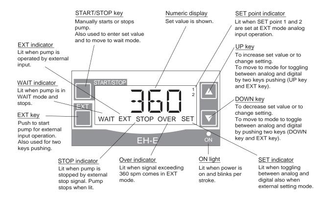
NOTE: Two keys pushing means to push simultaneously two keys of EXT key and UP or DOWN key.
