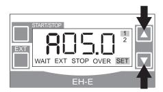
(5) Setting of input amperage at SET point 1. Set the input amperage at SET point 1 by ▲ and ▼ keys. The value increases with ▲ key pushed and decreases with ▼ key pushed. Amperage changes slowly by 0.1 mA when the key is pushed briefly, and changes quickly if pushed 3 seconds or more. Setting range is 0.0 - 20.0 mA.
