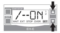
(4) Setting of pulse memory ON, OFF Push ▲ key and ▼ key to set ON and OFF of pulse memory. Display X -- ON shows the pulse memory ON and X -- OF shows memory OFF status. When the pump is shipped from the factory, it is set at / -- OF.
