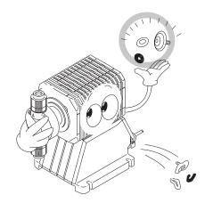
When you disassemble the pump head, replace diaphragm, O ring, valve gasket and valve unit by new ones.
