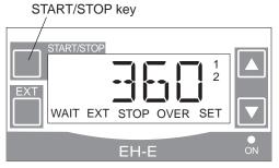
2) Push START/STOP key one time. The word WAIT disappears and pump starts operation. Every time START/STOP key is pushed, operation and stopping is repeated.
