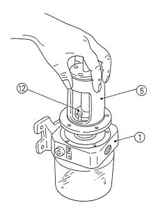
When the shaft has advanced to a position in which the flange surface of bearing housing [5] comes in contact with port housing [1], clamp them together by means of five hex socket head bolts [60] so that the drain is situated just below.
