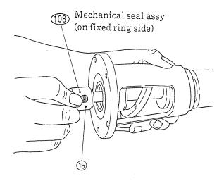
$\diamondsuit$  Position shaft [15] so that its shouldered surface is at the end of the retainer.
