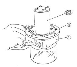
Remove five bolts [60] from the seal case unit on which the bearing holder unit is mounted, and detach the seal case unit from port housing[1]. Pull it out straight to prevent the end of the shaft of magnet capsule unit [104] from damaging the bearing in the bearing holder unit.
