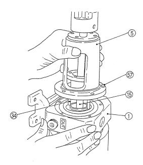
♠ Insert stud bolts [34] fixed to port housing [1] into two holes of seal case retainer
