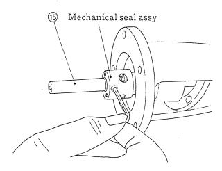
Carefully insert bearing housing [5] and end of shaft [15] into bearings [2] and [17] of port housing [1], and fix it by means of five bolts [57].
