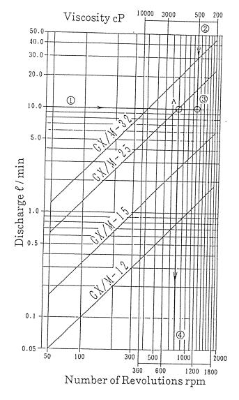
The performance chart shows discharges when the discharge pressure is  $0 \, \text{kgf/cm}^2$ .
