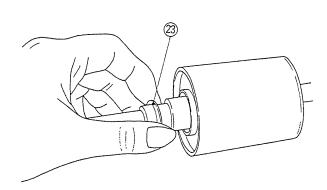
③ Press bearings [17] and [19] in slowly, rotating them gradually, until they come in contact with the side of shaft [15] provided with a key groove. Do this very carefully lest the bearings should break or fall.
