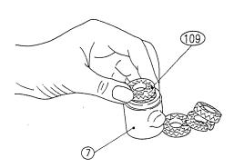
Attach gasket [38] to seal case [7] in which gland packing [109] has been loaded. Mount it on port housing [1] by using stud bolt [34] and seal case retainer [11] whose hole is positioned to the stud bolt and by loosening nuts [64].
