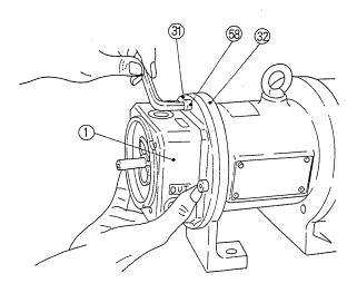
③ Detach sub-bracket [31] from port housing[1]. Take care not to scratch the surface of seal case [102].
