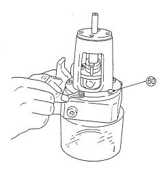
♦ Clamp two bolts [61] of packing retainer [12] alternately to prevent uneven clamping. To stabilize gland packing [109] in seal case [7], first clamp them lightly by means of a wrench or similar tool, loosen them again, and reclamp them tightly by hand.
