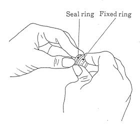
② Fit the fixed ring of the mechanical seal assy into seal case [7]. At that time, position the notch in the fixed ring to spring pin [54] of the seal case assy and insert the fixed ring until it comes in contact with the deep end of the seal case. Take care that the sliding surface is not scratched during insertion.
