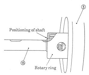
Clamp two set bolts of the mechanical seal assy to fix it to shaft [15].
