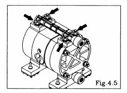
• Remove the 4 retainer nuts from the out manifold, and remove the out manifold. [Fig.4.5]
