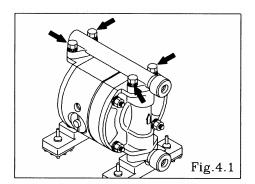
• Remove the 4 retainer bolts from the out manifold, and remove the out manifold. [Fig.4.1]
