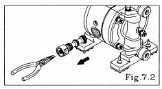
• Draw out the C spool valve assembly using the plyer, and remove the seal ring from the C spool valve assembly. [Fig.7.2]
