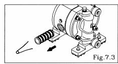
• Remove the sleeve using the sleeve remover (special tool: Part number 713148). [Fig. 7.3]
