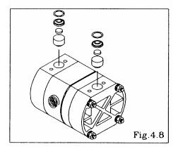
${\ }^{\bullet}$  Remove the O ring, valve seat, flat valve and valve stopper. [Fig. 4.8]
