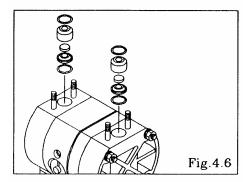
$\bullet$  Remove the O ring, valve stopper, flat valve and valve seat. [Fig.4.6]
